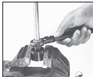
Step 7 – Hold tube steady against internal shoulder of Ferulset Tool or fitting body and tighten nut an additional 1-3/4 turns.
